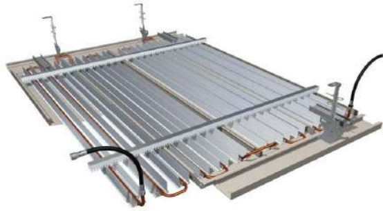
Figure 3.3. Example of a cooling panel (Babiak et al., 2009).
